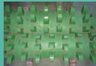
36x48 Tooth plates after renovation
